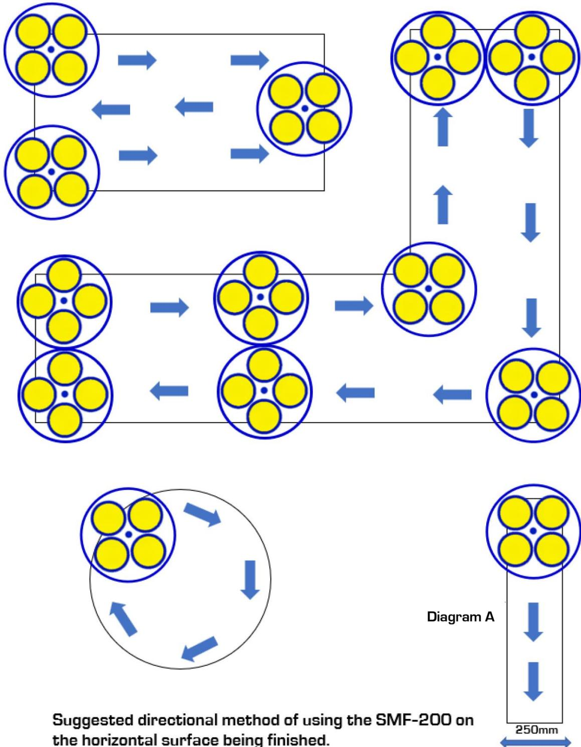
**Suggested directional method of using the SMF-200 on the horizontal surface being finished.**
